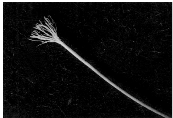
Figure 4 Fibrils in PP/PVAc blend fiber.
